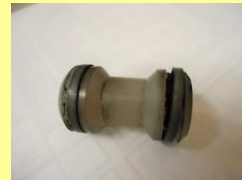
Parts worn out by no lubrication
